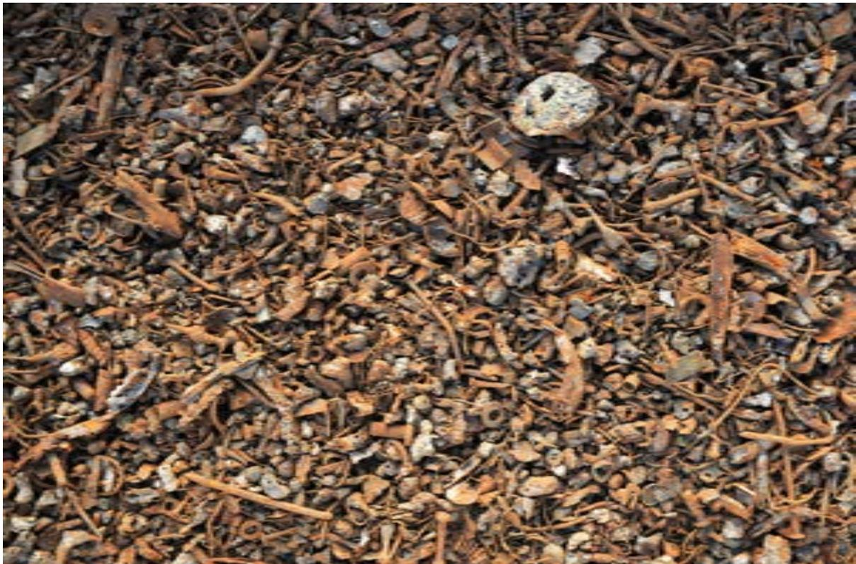
*Ferrous metal after processing and sorting*
